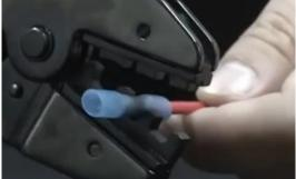
copper in the connector is joint tightly.
